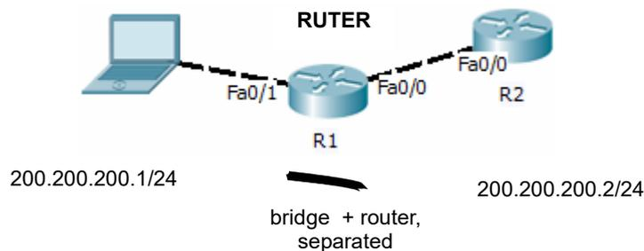
Check the communication between PC and router R2 (ping) via the CRB bridge.
