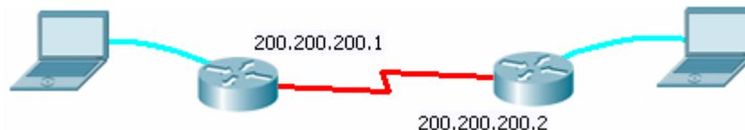
2. In each of the routers a serial select the interface to configure. The name of interface is dependent on device's installed expansion cards and base interfaces present. These are, for example: serial 0/0 or s 0/0:
