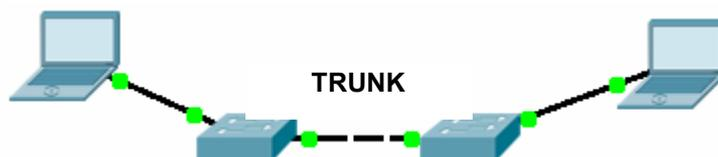
3. In both switches configure ports leading to another switches as trunk ports (in the example is fa0/1)
